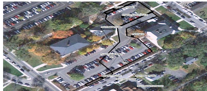
Area of the design site parking lot considered in the SWMM mode
